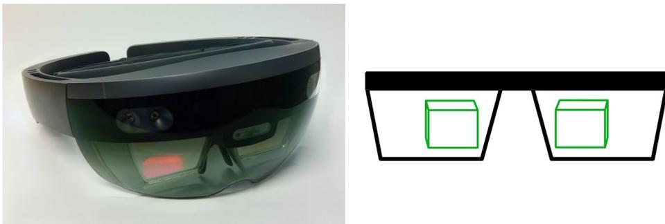
**Fig. 1** The left side shows a photo of the HoloLens. The right side demonstrates how a green cube is projected onto the glasses of the HoloLens. Projecting different perspectives of the cube on each of the glasses creates the illusion that a 3D cube is floating in front of the user
